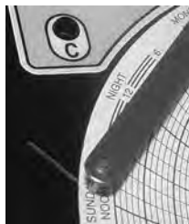
Chart recorder stylus and time line groove
