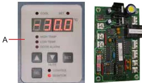
Left: Horizon display with touchpad. Right: Rear view of display showing monitor/control board.
