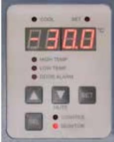
Horizon Series monitoring and control system display.
