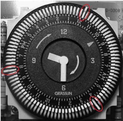
Horizon Series defrost controller with defrost times set to On position at 12:00 AM, 8:00 AM, and 4:00 PM.
