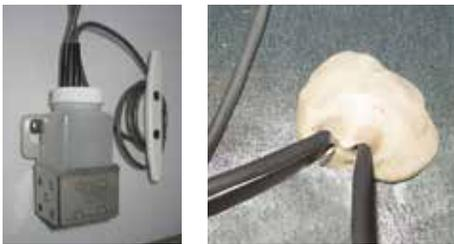
Left: Probe bottle with temperature and chart recorder probes. Right: Access port on the top of the freezer. The number and location of ports varies by model.
